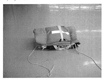
4.2.1.13 Pass a length of black 1.4mm polyester cord (Art no. 0.04.01.09.0) around the folded liferaft and secure it *tightly*.
